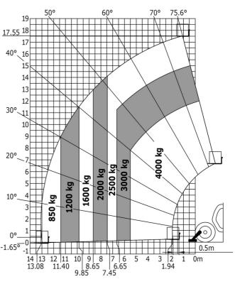
Machine on stabilisers with Man basket Metric
