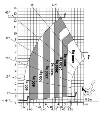
Machine on lowered stabilisers with forks Metric
